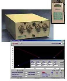
The Q-Grad Pump provides high-pressure quaternary gradients for HPLC applications. Four high-performance pumps are packaged into a single cabinet and are controlled with PC-driven software. The result is high-pressure gradient capability that is as economical as low pressure mixing systems.
