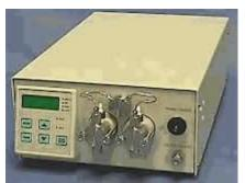
The Series 1500 Constant Flow Pump has been designed for analytical to small-scale preparative chromatography applications. The patented low-dead-volume pulse damper and dual piston mechanism make this pump virtually pulse-free, and provide unmatched performance for the most demanding applications. The unit provides constant flow rates from 0.01 to 12.0 ml/min and is typically suitable for columns from 2mm up to 22mm ID.
